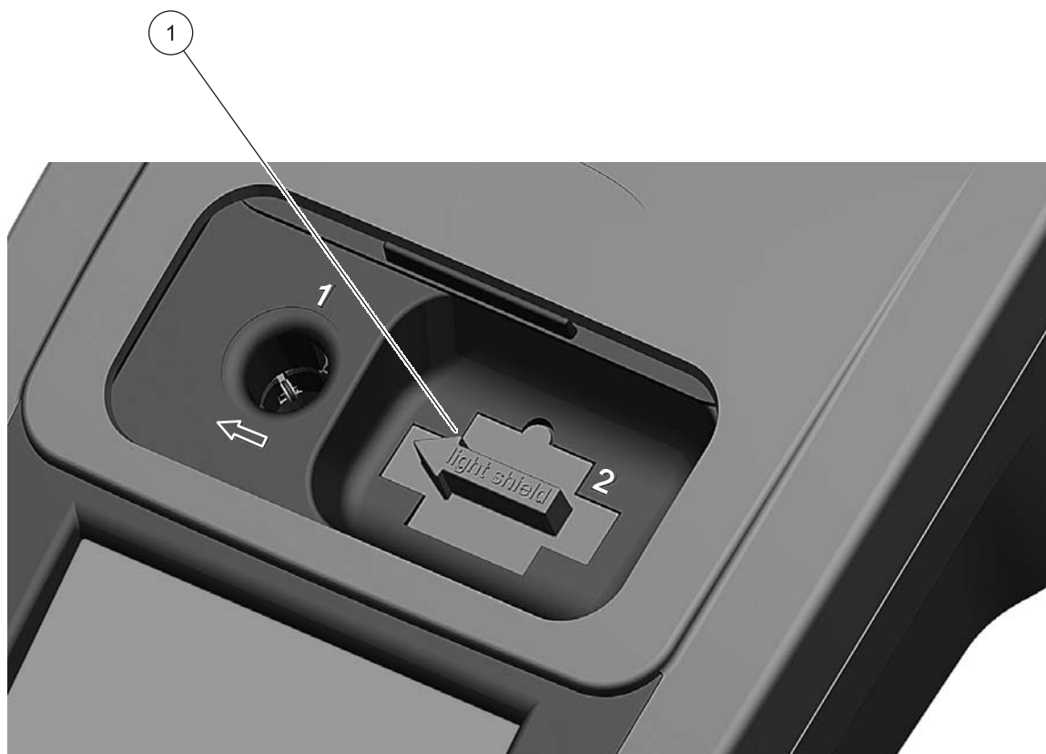
Figure 6 Light Shield in place
